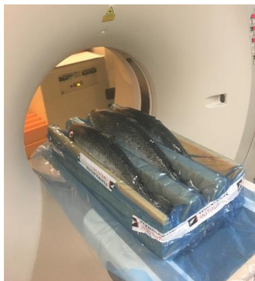
Figure 6 Fixture made in foam (Sundolitt). This type of fixture was used in CT scanning of dead fish and was further developed for the needs of live fish scanning.
