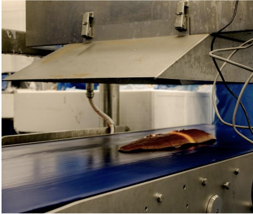
Figure 22 Qvision measurement of salmon fillets during the first trial.
