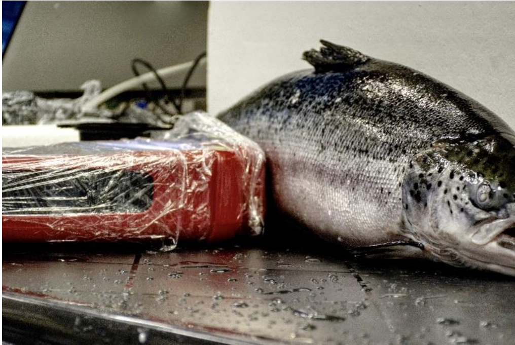
Figure 24 Measurement of pigmentation from whole dead fish with handheld SORS instrument.
