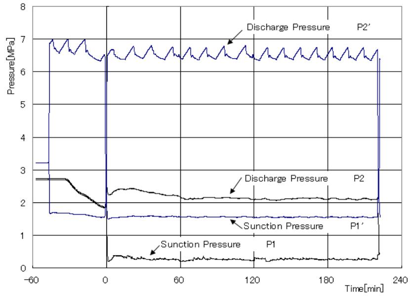
**Fig 12.** Variations of measured CO<sub>2</sub> pressures of HTC and LTC with time.
