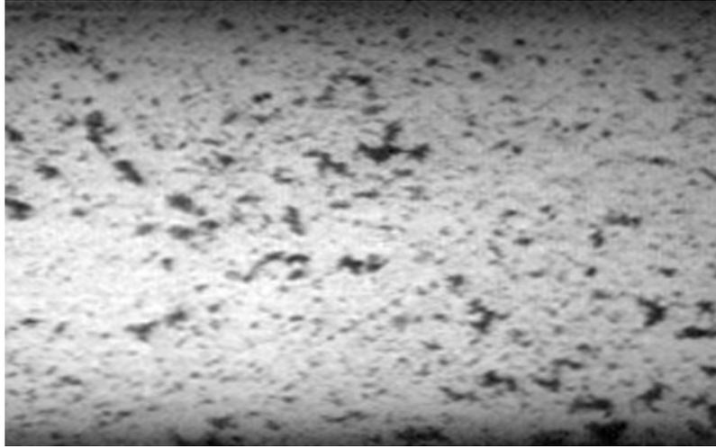
(a) CO<sub>2</sub> solid-gas flow at opening conditions of 15mm of expansion valve
