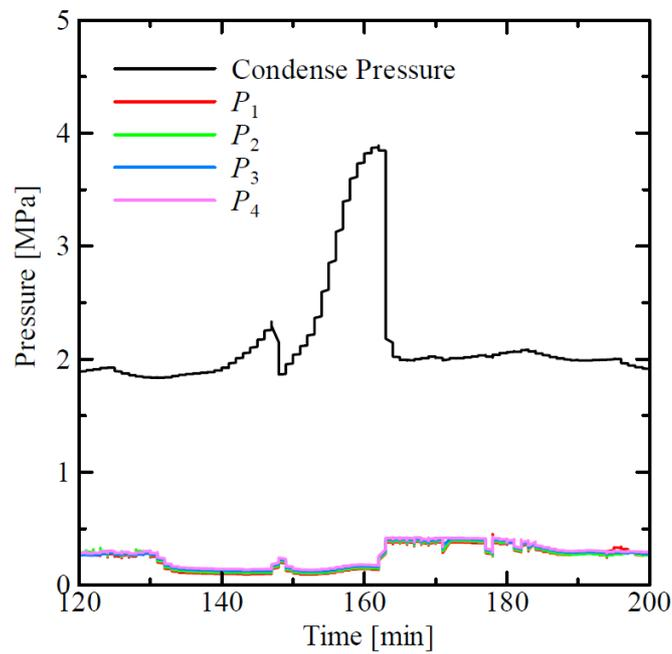
**Fig 7.** Behavior of measured condensing and local pressures in test section at expansion valve opening 10mm, condensing temperature -20°C and heat input 900W
