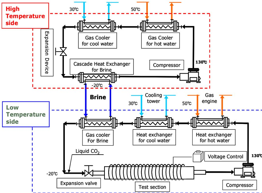
Fig 1. Schematic of the CO<sub>2</sub> cascade refrigeration system
