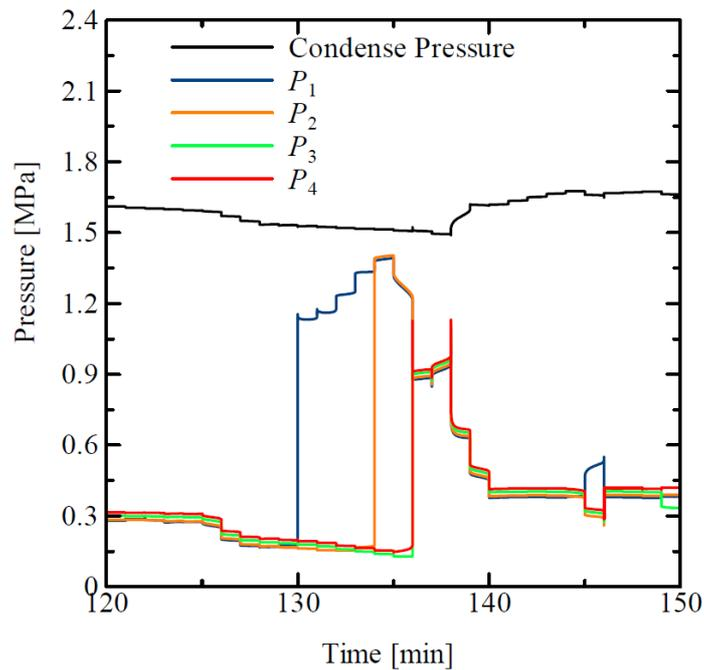
**Fig 9.** Behavior of measured condensing and local pressures in test section at expansion valve opening 15mm, condensing temperature  $-25^{\circ}\text{C}$  and heat input 1200W
