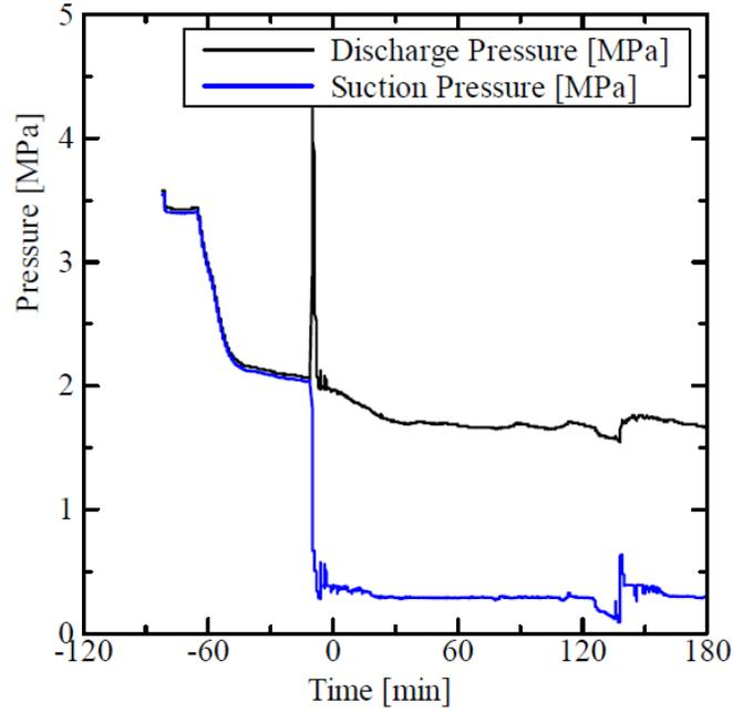
**Fig 8.** Measured suction and discharge pressures in LTC vary with time (the expansion valve opening in 15mm, the condensing temperature of  $-25^{\circ}\text{C}$  and the heating power input 1200W).
