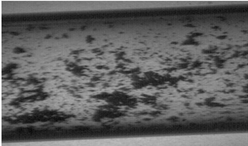
(b) CO<sub>2</sub> solid-gas flow at at opening conditions of 10mm of expansion valve
