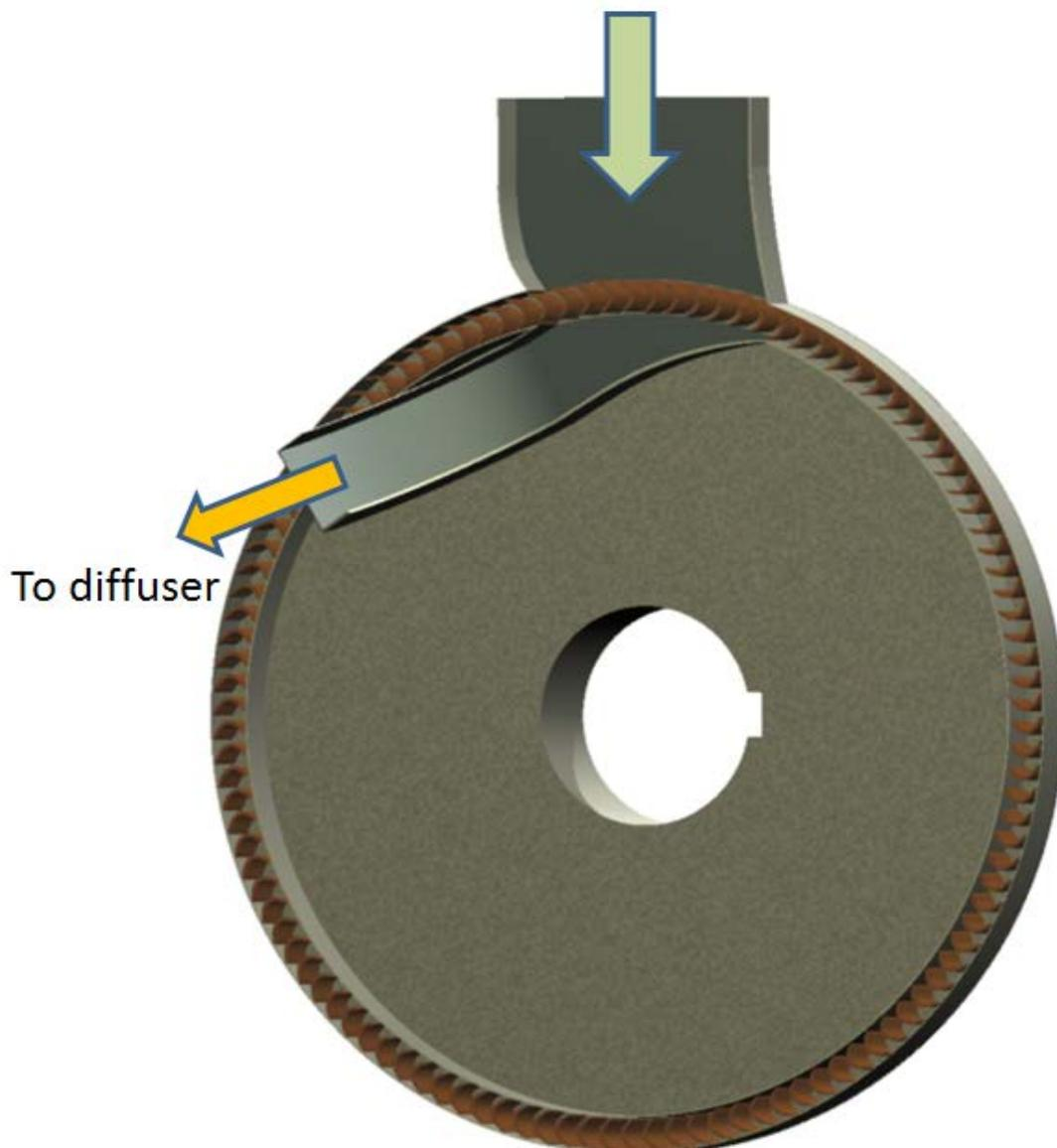
Figure 7. The concept of the partial admission CO<sub>2</sub> turbo-compressor
