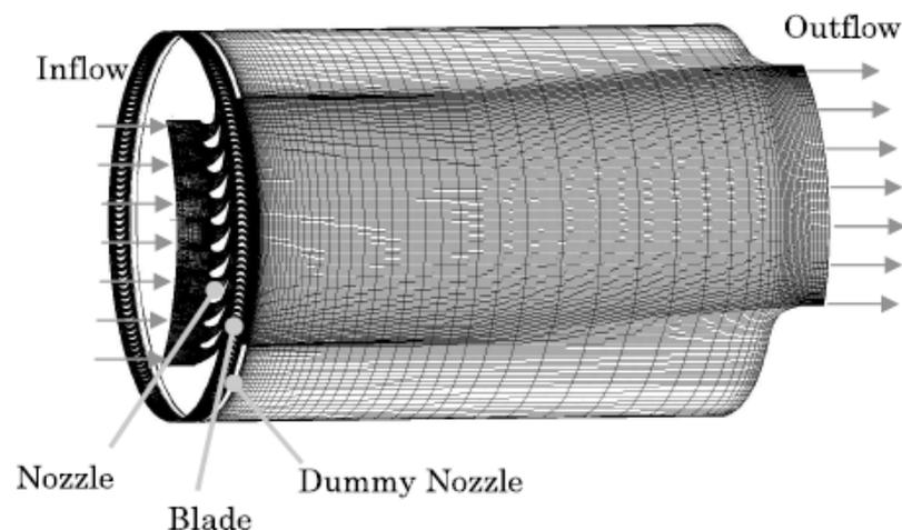
Figure 1. Numerical grid for simulation of partial admission axial steam turbine. Source: Sakai et. al.
