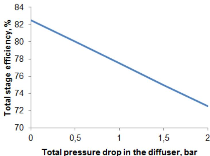
Figure 11. Stage efficiency vs diffuser total pressure drop
