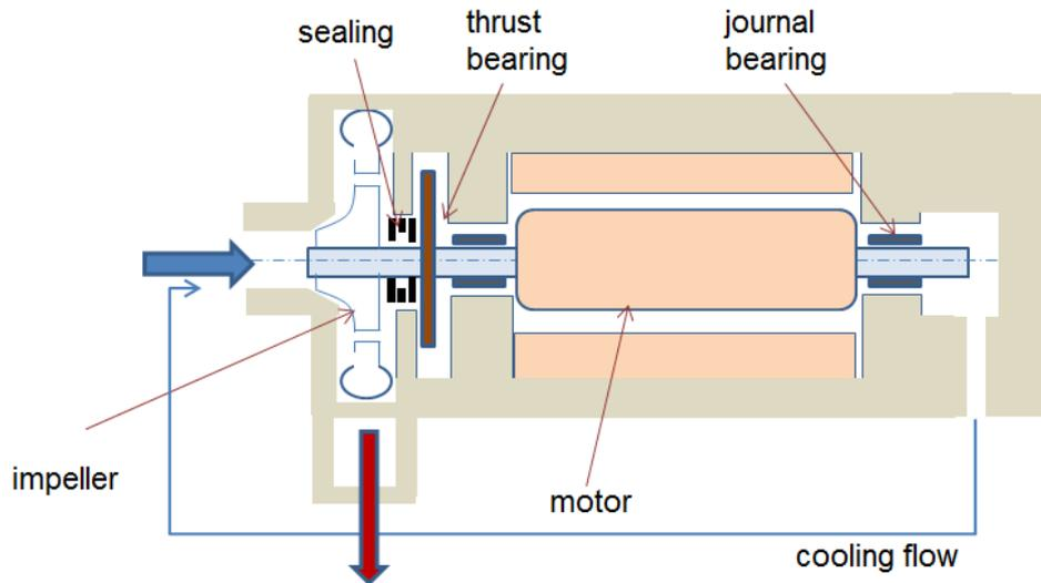
Figure 4. The reference compressor concept
