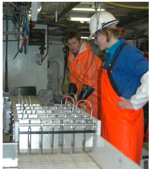
Improved catch handling on board by electrical stunning.
