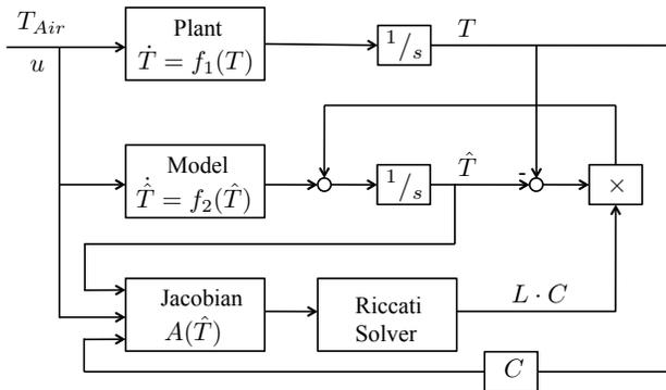
Fig. 3. Design schematic
