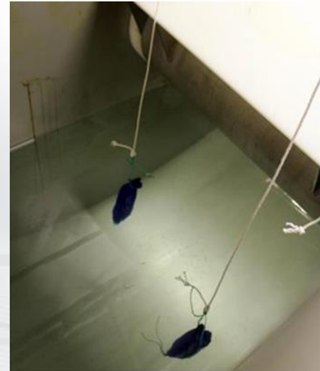
Logging temperature in bleeding tank
