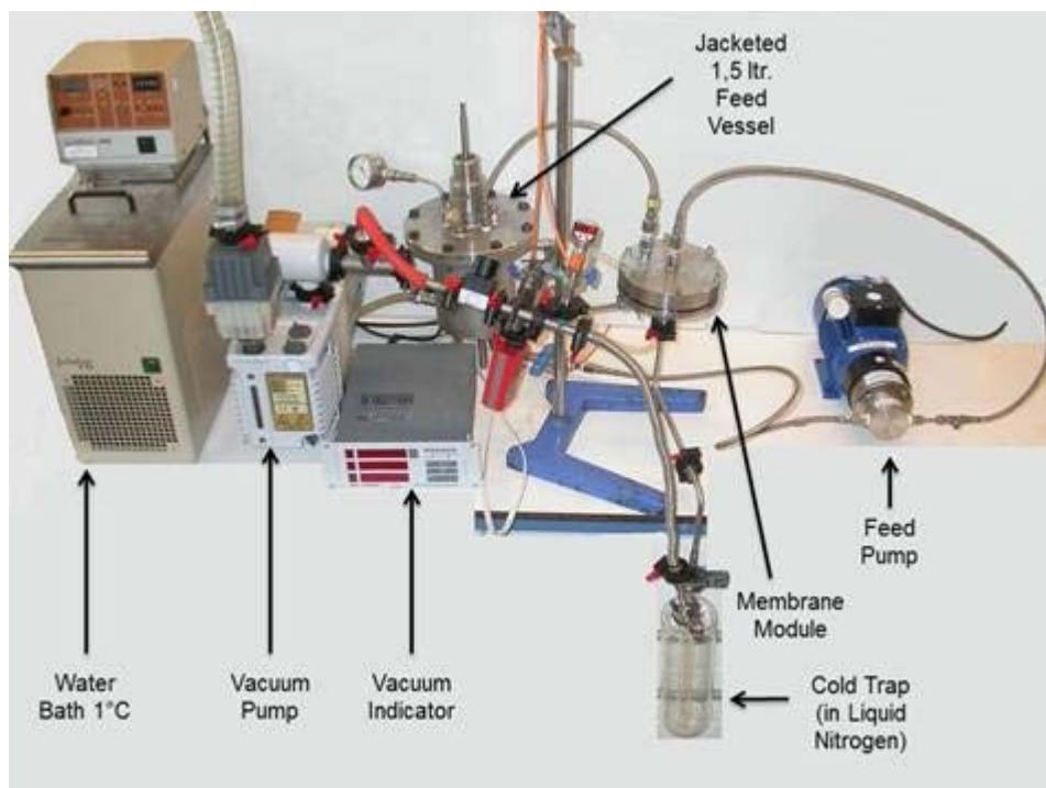
**Figure 1:** Set up of the PerVaporation process. The Fish extract was pumped over the membrane back to the feed vessel. At the permeate side of the membrane the volatiles were condensed in the cold trap in liquid nitrogen under vacuum.
