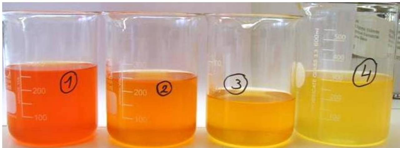
**Picture 4.** Ethanol fractions after each of 4 steps of ethanol extraction of the dried washed sediments.
