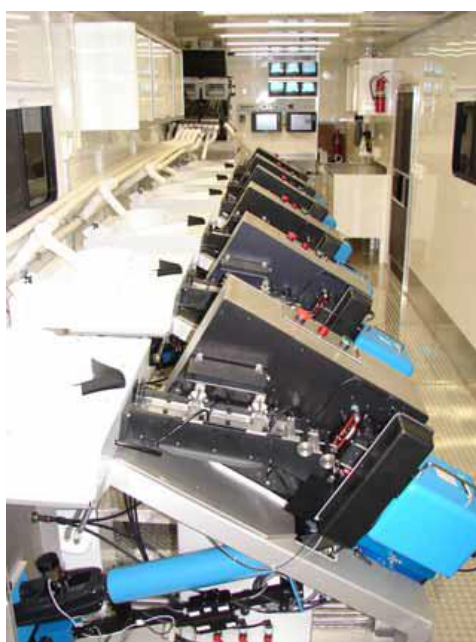
Figur 16 AutoFish System installert i trailer
