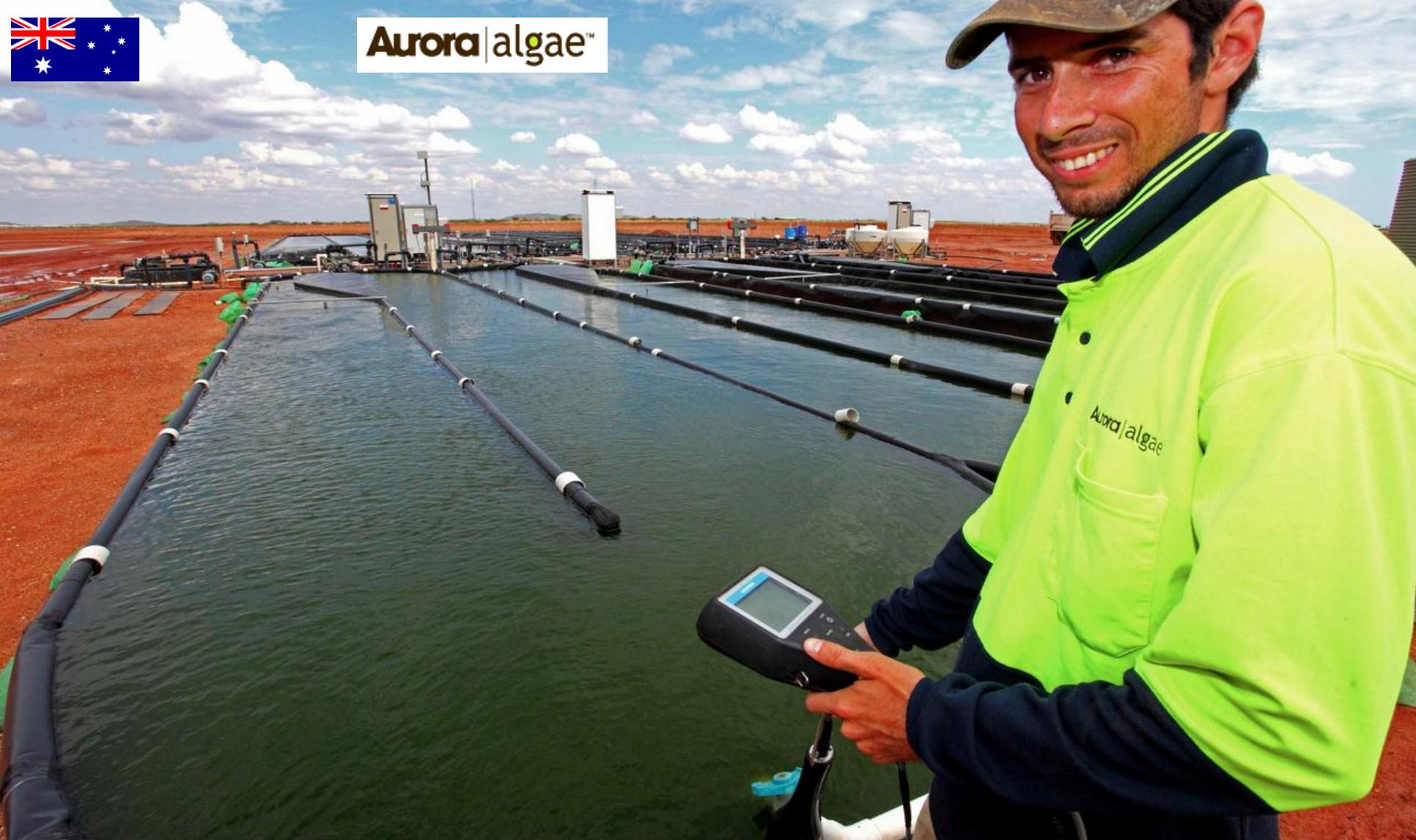
Aurora has combined traditional techniques with modern control systems technology to achieve maximum productivity in large-scale operations. All operations, from growing to harvesting biomass, are automatically controlled. The system measures variables such as temperature, pH levels, and turbidity and initiates adjustments as necessary. Information is instantly captured and available to the R&D team to allow further improvements and increased productivity.
