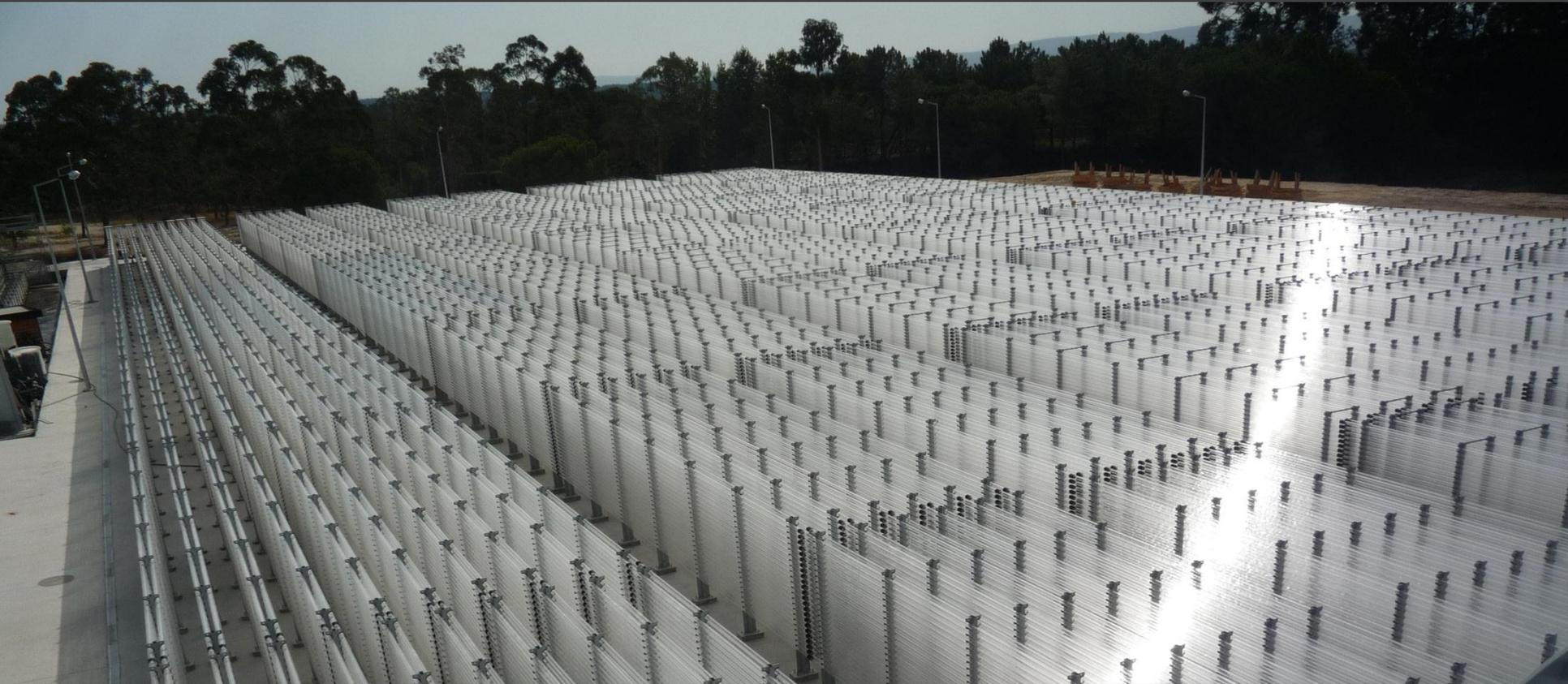
The unit will have a total 10.000 m<sup>2</sup> area, and will work with more than 1300 m<sup>3</sup> volume of production photobioreactors, being the world's largest unit of microalgae production with closed photobioreactors.
