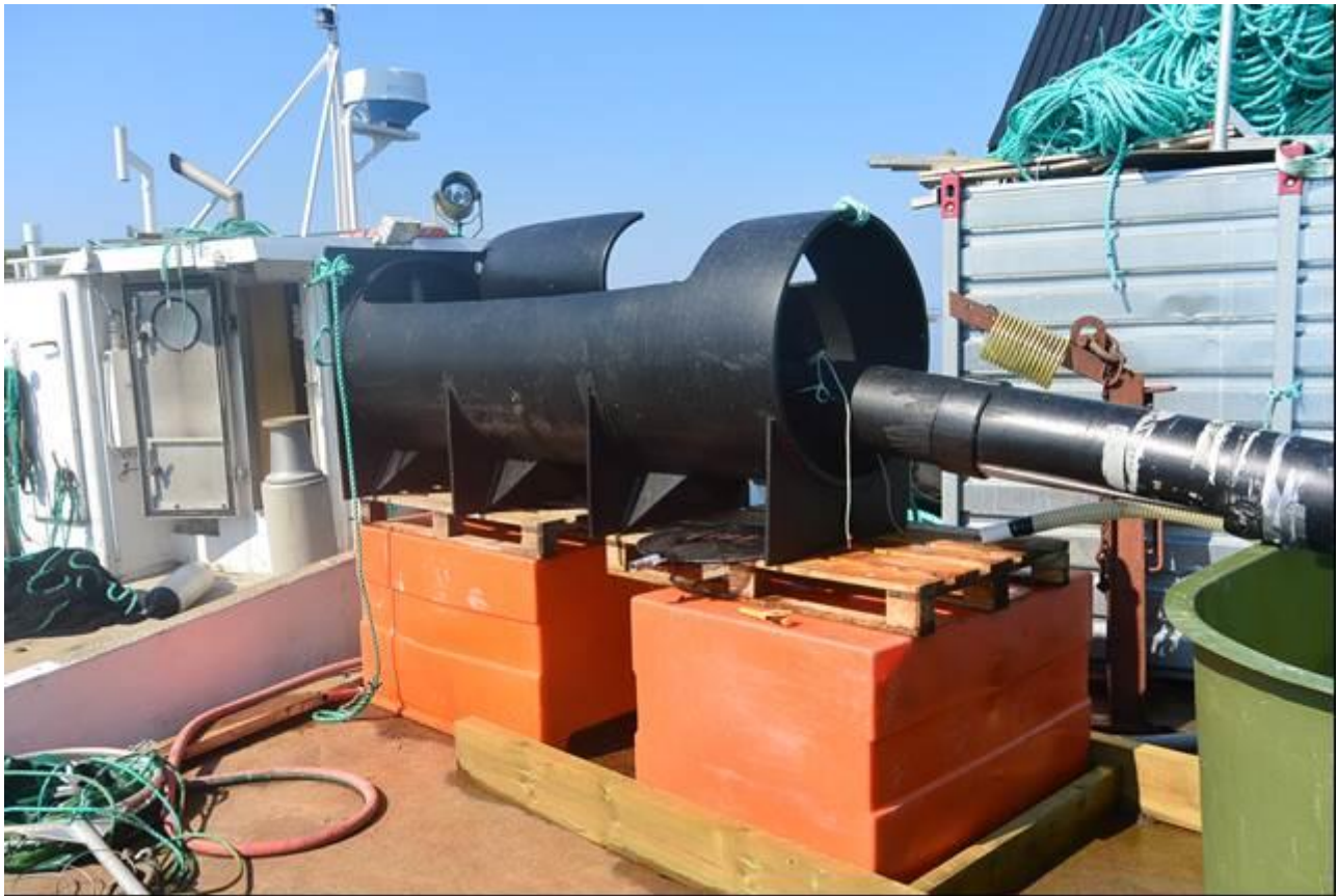
Picture 2 The holding tank used to transfer the fish from the cage to the freshwater tank. The pipe has slits at the bottom to prevent seawater entering the holding tank.
