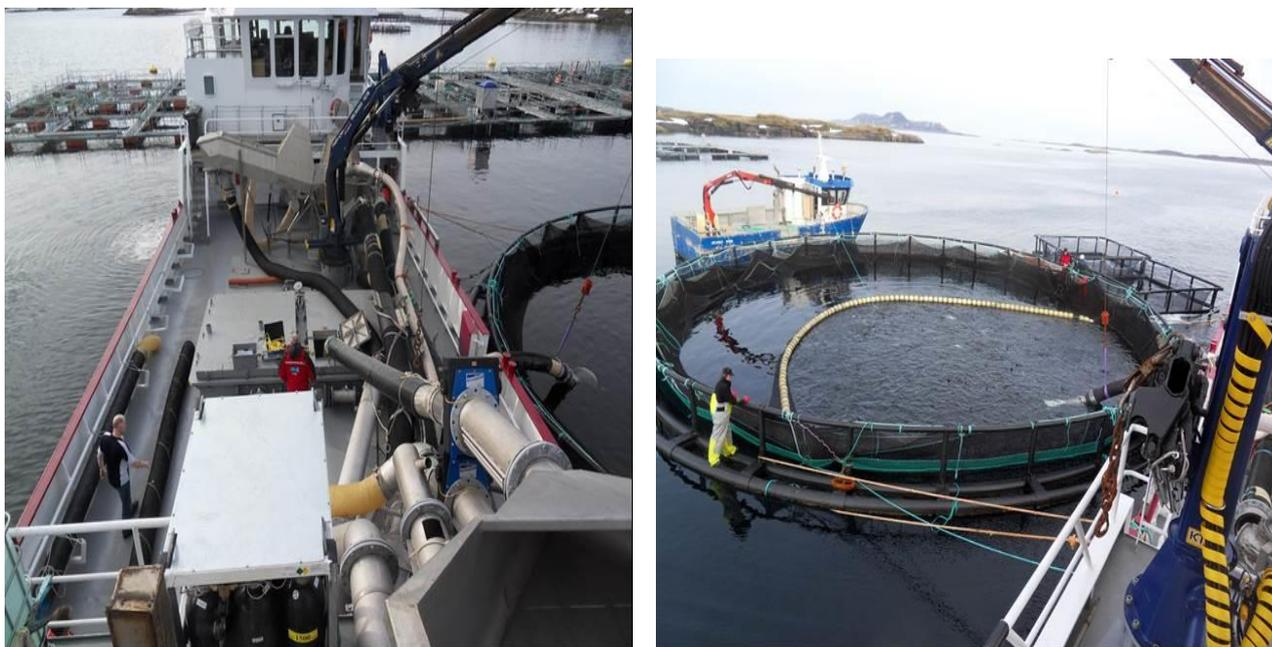
**Figure 1.**The well-boat used in the study and fish being pumped from the polar circle into the two wells on board.
