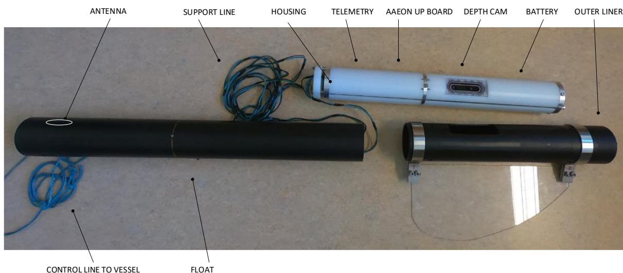
Figur 8 –Oversikt over deler i Stereo-Catch Monitoring Proben (S-CMP) .
