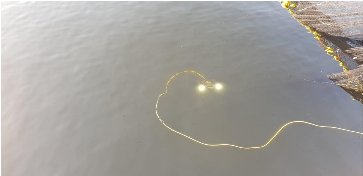
Figure 18 - ROV ("FishBot") inside purse seine with lights on.
