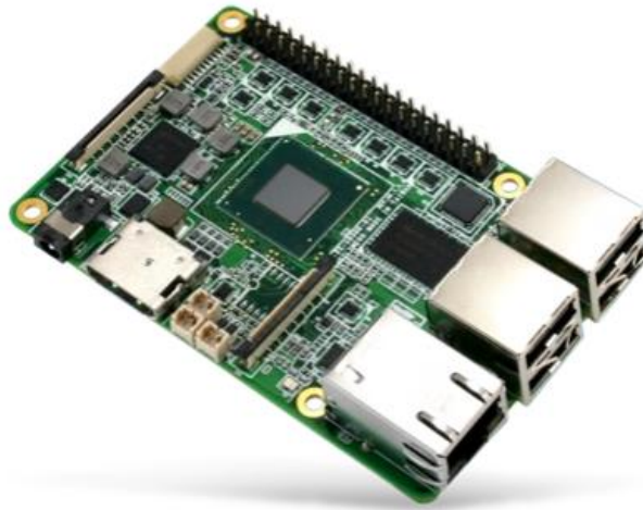
Figure 10 - Image of AAEON UP board. [Image: up-board.org]
