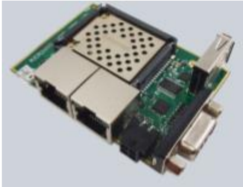
Figure 11: Microhard pMDDL2450 with motherboard [Image: Microhard]
