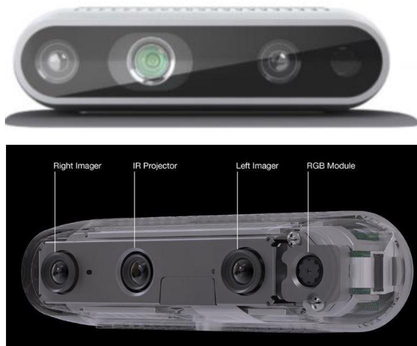
Figure 1 - the Intel RealSense Depth Camera D435i. [Image: Intel].
