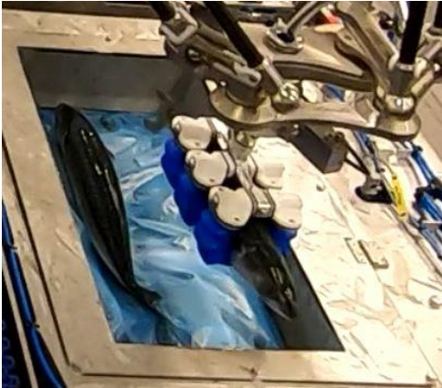
Automated layering of plastic for a completely automated packing process
