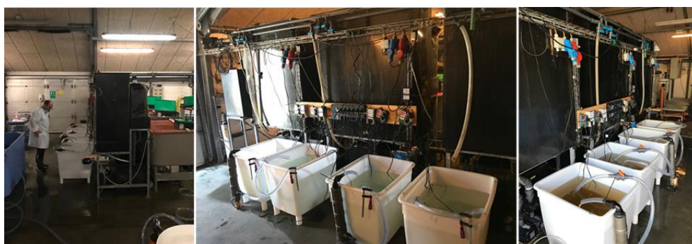
Figure 1. Test of PAA degradation in clean freshwater and seawater (left) with and without UV. PAA addition with and without UV were tested in mature RAS water.
