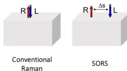
Figure 23 A general schematic description of the optical configuration of conventional Raman spectroscopy (left) and SORS (right), respectively.
