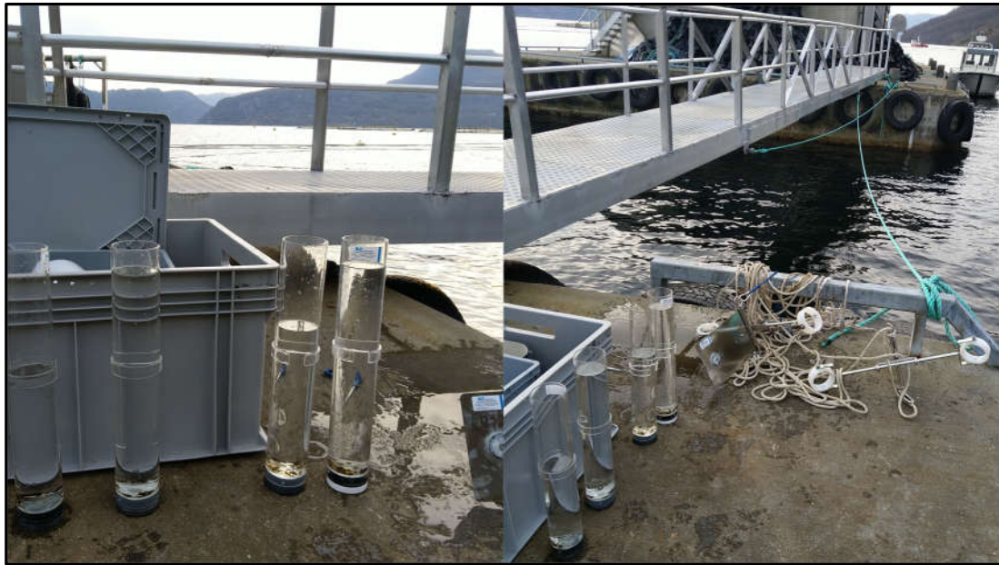
Figure 2.12 – Deployment of sediment traps (two chambers for each depth) at the reference site.
