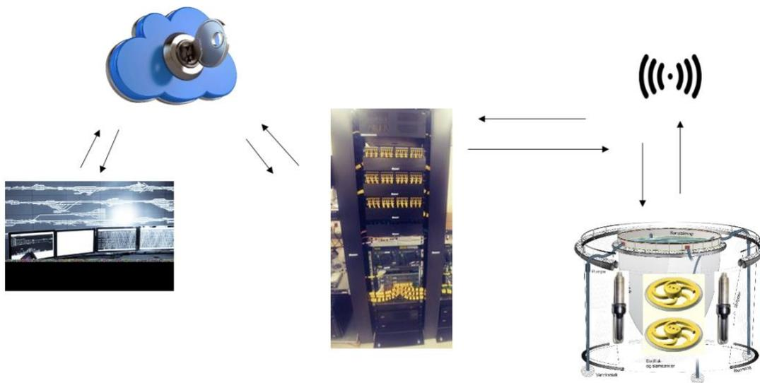
Figure 7. The AcuLice system consists of a central control room with monitoring, an electronic processor located on the facility and a component in the sea (that sends out low frequency sound waves). The whole system is connected to internet.
