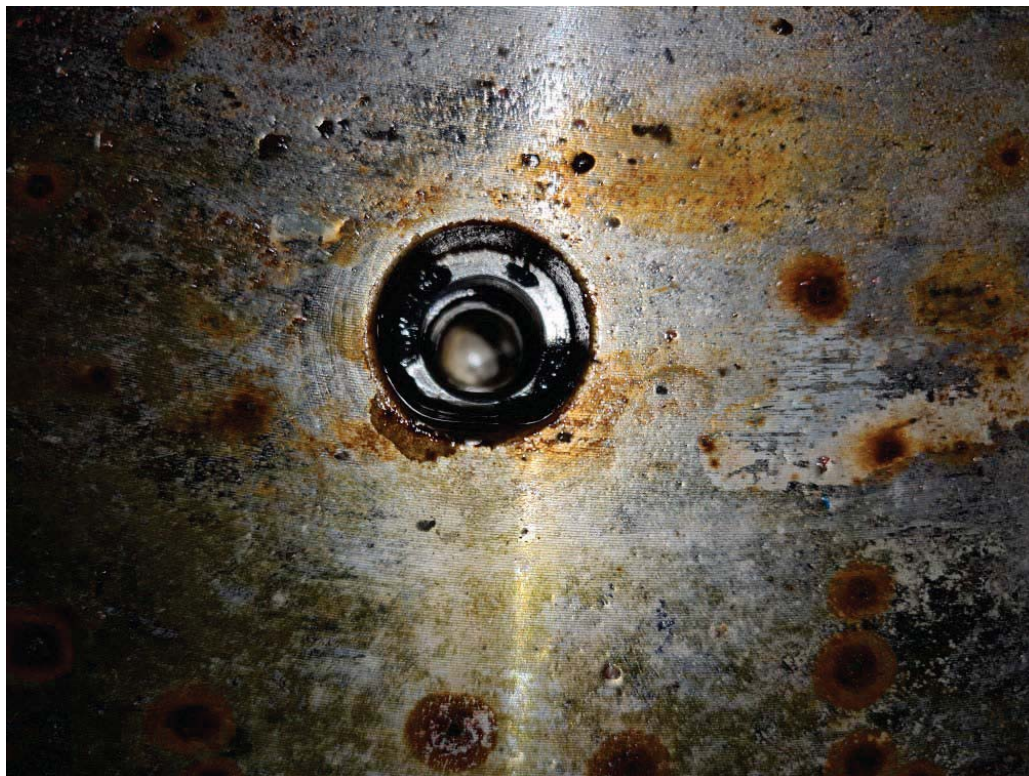
Figur 12. Korrodert skru hull i kapsel for propellhode
