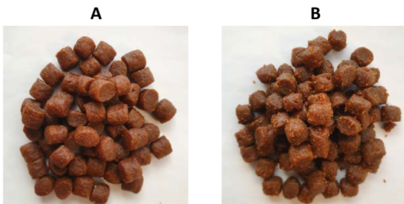
Figure 12: Photographs of fresh (unused) pellets (A) and used pellets taken out of the pneumatic conveying test rig after finishing all pressure tests (B).
