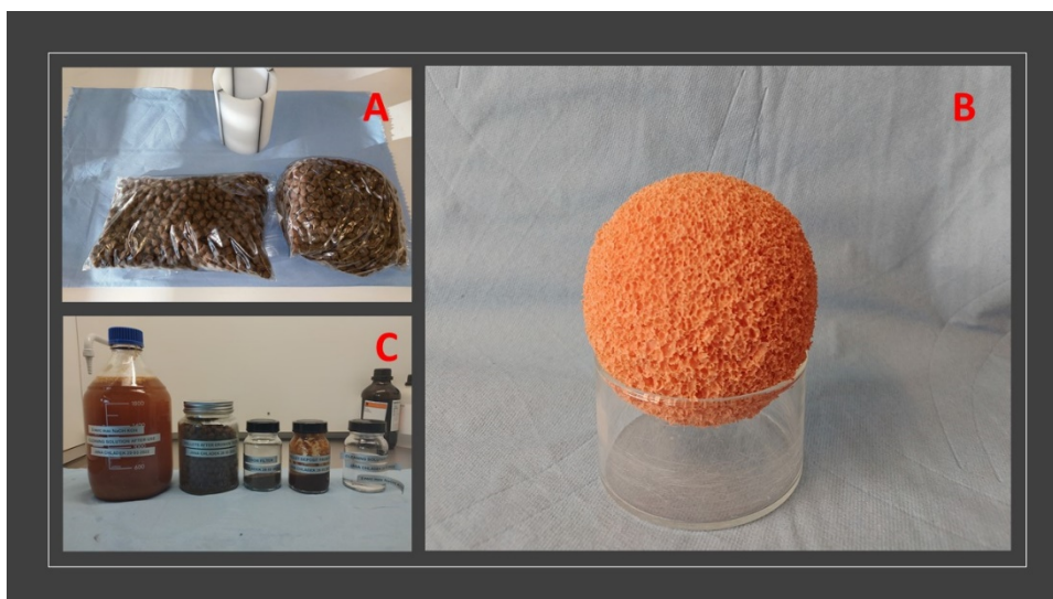
Figure 20: Testing material received from WP1. A) Pristine fish feed pellets and a sample of the feeding hose used within the convey pilot test; B) Sample of the cleaning sponge kindly provided by AKVA Group; C) samples collected from both different areas in the pellets conveying system and steps in the simulation process.
