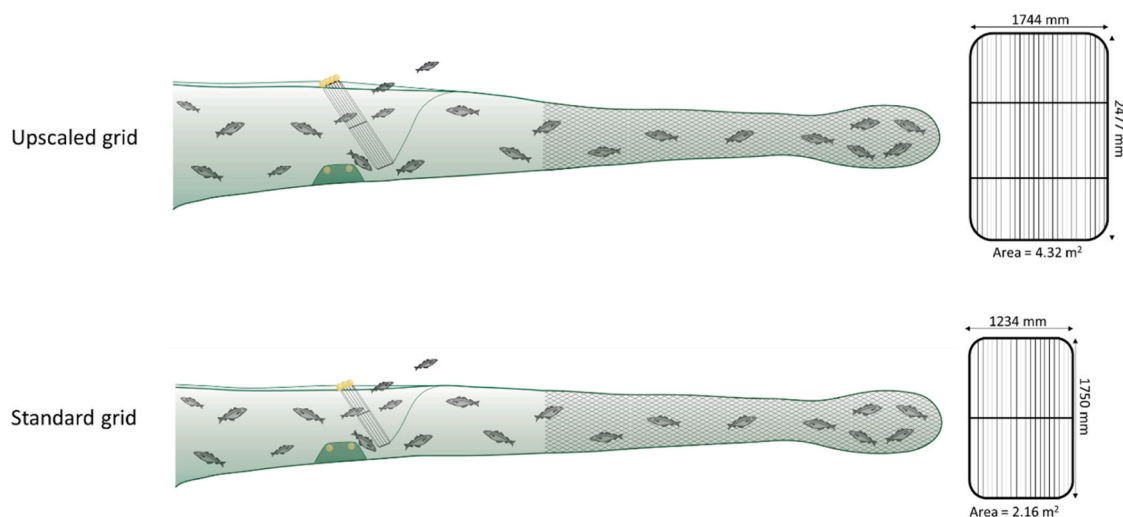
Fig. 2. Illustration of the gear configuration used during the trials with the upscaled and standard grids.
