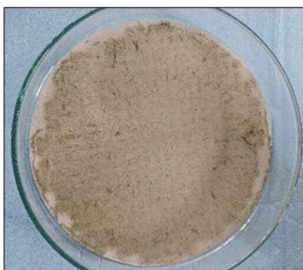
Figur 7. Sample of filter obtained from the laboratory based net cleaning simulation.
