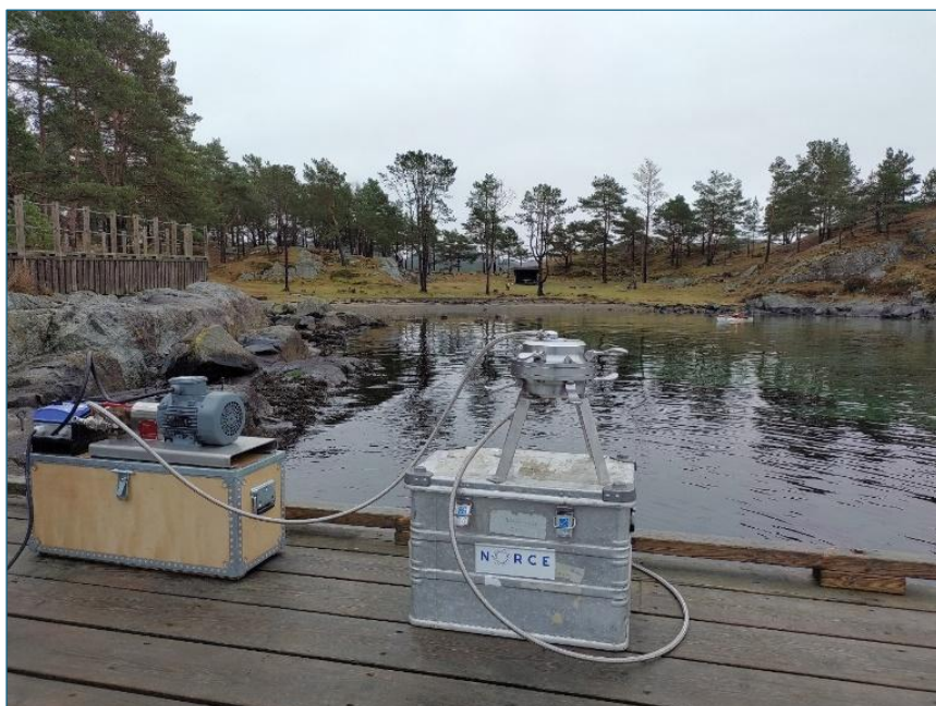
Figur 6. NORCE engineered MPS sampling device.
