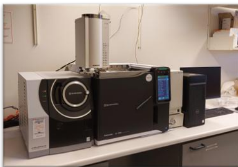
Figur 9. Pyr-GCMS equipment at NORCE Mass Spectrometry Lab (Photo: Adrián Jaén-Gil, NORCE).
